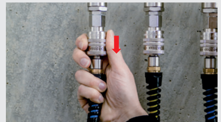
Disconnection - second step: Safe decoupling
