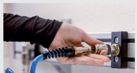
Disconnection: Separate the coupling from the plug after loosening the locking nut
